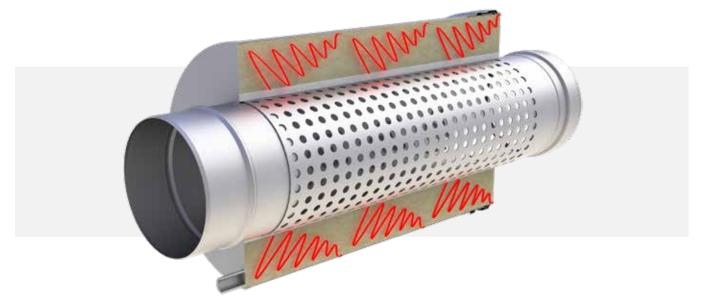
All Jeremias absorption silencers are filled with non-combustible mineral wool. In order to protect these from fiber discharge by the exhaust gas flow, a protective fleece is often incorporated between the perforated sheet metal and the mineral wool. Depending on the composition of the exhaust gases and the operating conditions, different materials are used to protect the mineral wool:
