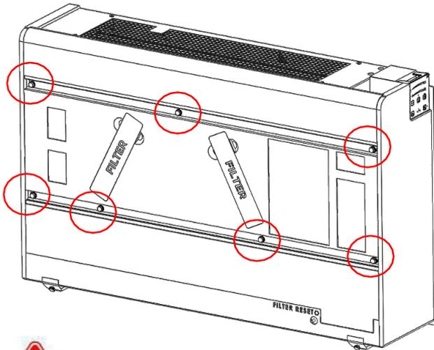
**2****ÖFFNEN SIE DEN DECKEL DER EINHEIT, UM ZUGANG ZU DEN INTERNEN KOMPONENTEN ZU ERHALTEN**
